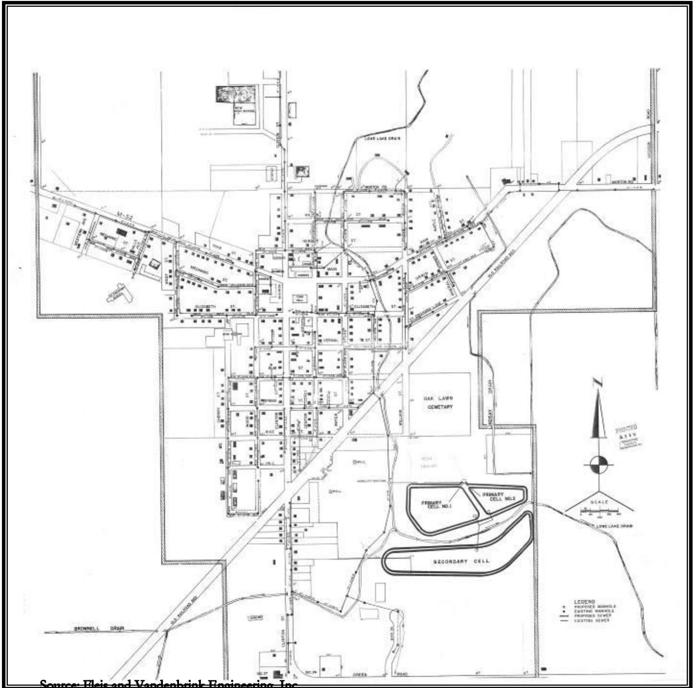
FIGURE 5 VILLAGE OF STOCKBRIDGE UTILITIES SEWER LINES
